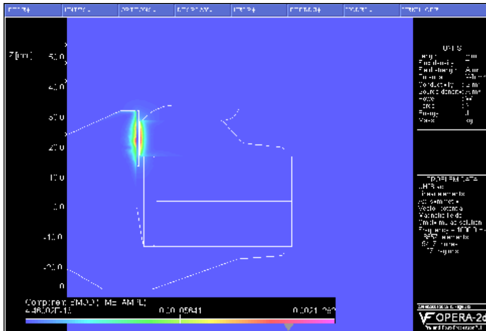
Figure 10. Contour Plot of the Induced AC Magnetic Field, |B(r,z)| , for the Over Hung Motor Assembly at 1.0 kHz with 1.0 A Input.
