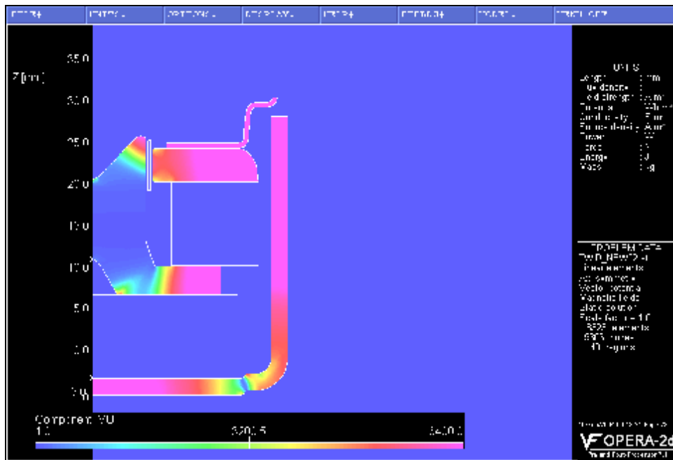
Figure 21. Contour Plot of the Relative DC Permeability for the Restart Nonlinear AC FEA Solutions for the New Motor Assembly.
