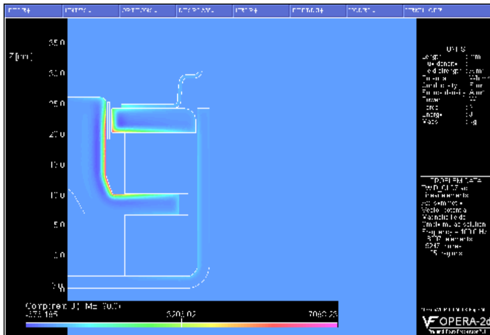
Figure 15. Contour Plot of the Induced Eddy Current Density in the Old Motor Assembly at 100 Hz.
